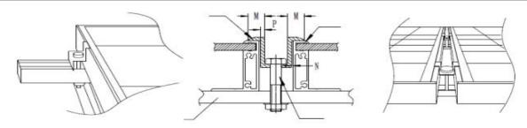
Dimension "M" represents the mounting overlap dimensions for clamp and moudule frame fronts;
