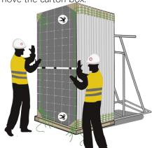
④ Cut off all the horizontal packing belts. When there are 1-2 vertical packing belts remaining, push the module gently to tilt toward the stand supporter.
